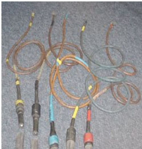
Photograph No. 7, showing examples of ‘single core’ cables with ‘open tails’ to make the connections to a supply
